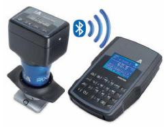
Wireless tester's version with embedded display and bluetooth support console.
