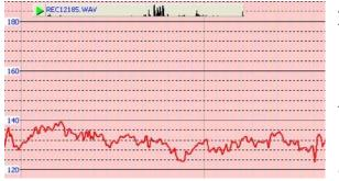
Audio notes dictated during measurement or longterm recordings are shown in the diagram directly at the corresponding point of dictation.
