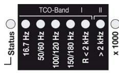
The frequency-LEDs change their colour in proportion to their contribution to the total field strength. See below for details on LED display modes.
